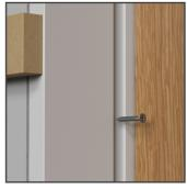
The doorset is secured into the opening by fixing three screws into the lining next to and three opposite the hinges. Two further screws should be fixed into the head.
