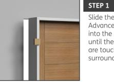
Slide the Simpli Advanced doorset into the opening until the fitting pads are touching the surrounding wall.
