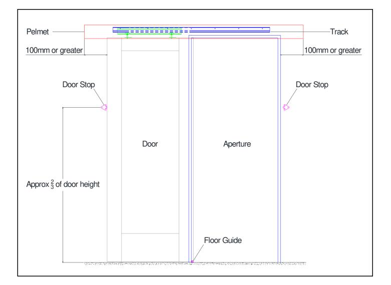
Mark the Hangers location centrally, 430mm apart from the centre of the door's top edge. Pre-drill the Hanger bolts.
