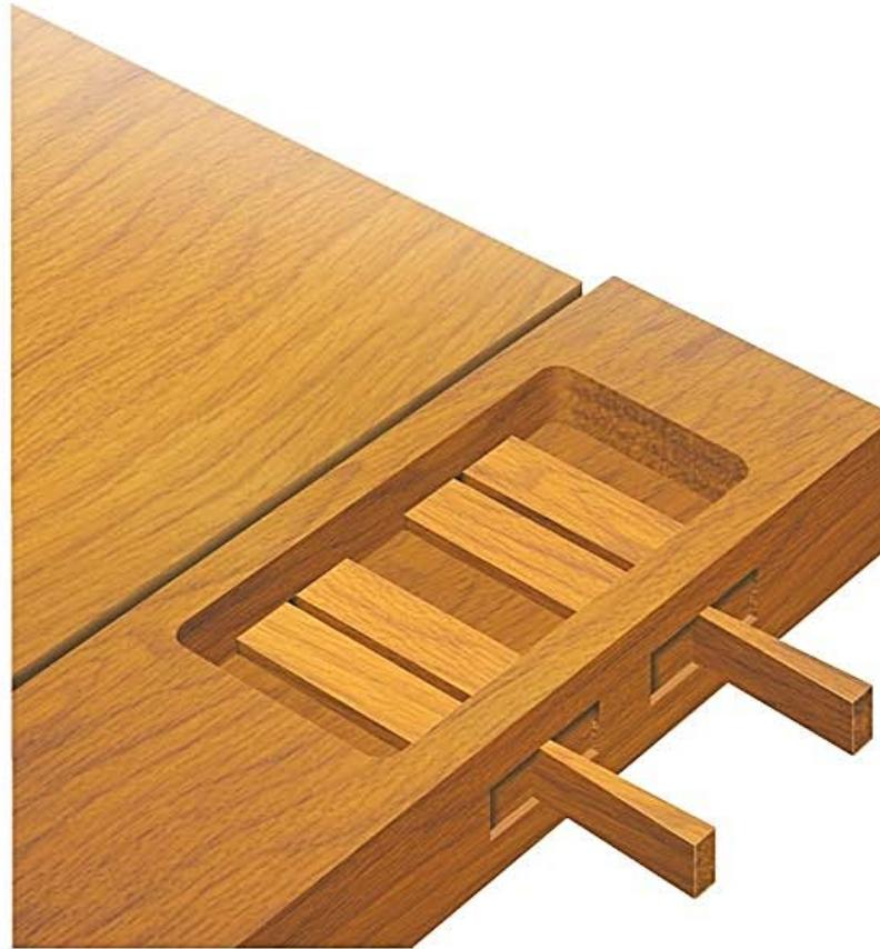
M&T = "Mortice & Tenon", method of joint construction
